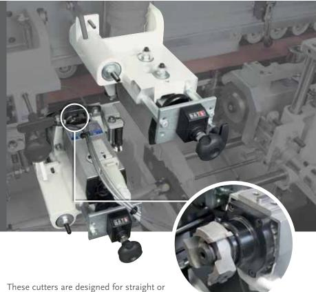
These cutters are designed for straight or radius trimming of any type of edge, whether it is thick or thin, made of PVC, ABS, melamine, laminate or wood. The edge thickness is easily set by means of two numerical readouts.
