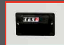
digital readout for the fence position on the parallel fence It allows precise positioning with the magnetic strip sensor.
