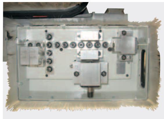
**Boring unit with 12 vertical spindles
