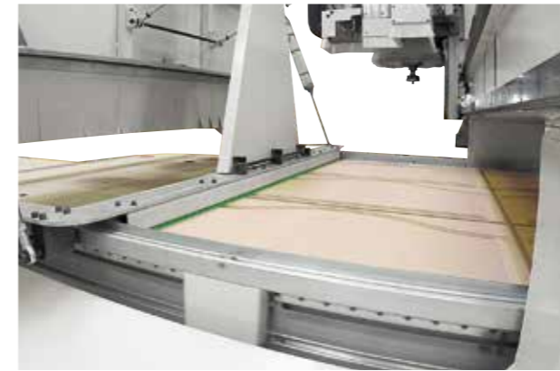
100% productivity with the pusher that moves the processed work pieces on the unloading belt and simultaneously cleans the work table while the new panel to be machined is loaded.
