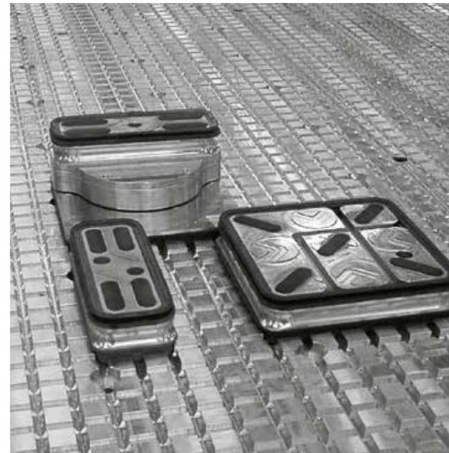
Any machining process without removing the spoilboard and no obstacles thanks to the tubeless X-PODs.
