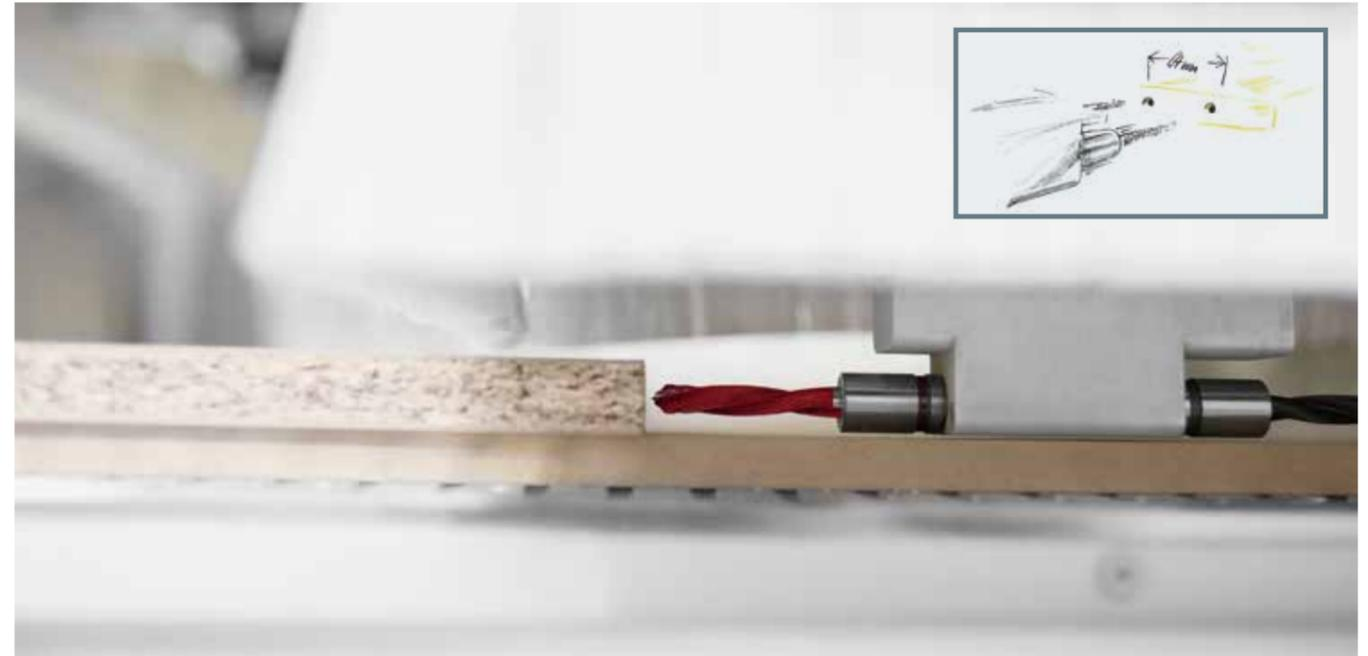
HINGE UNITS: THREE DRILLS IN ONE STEP!
