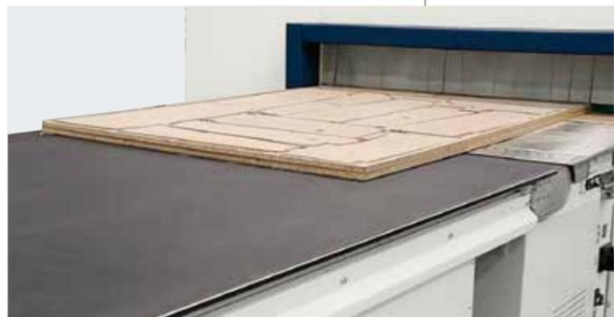
High productivity: the pusher moves the processed work pieces on the unloading belt and simultaneously cleans the work table while the new panel to be machined is loaded.
